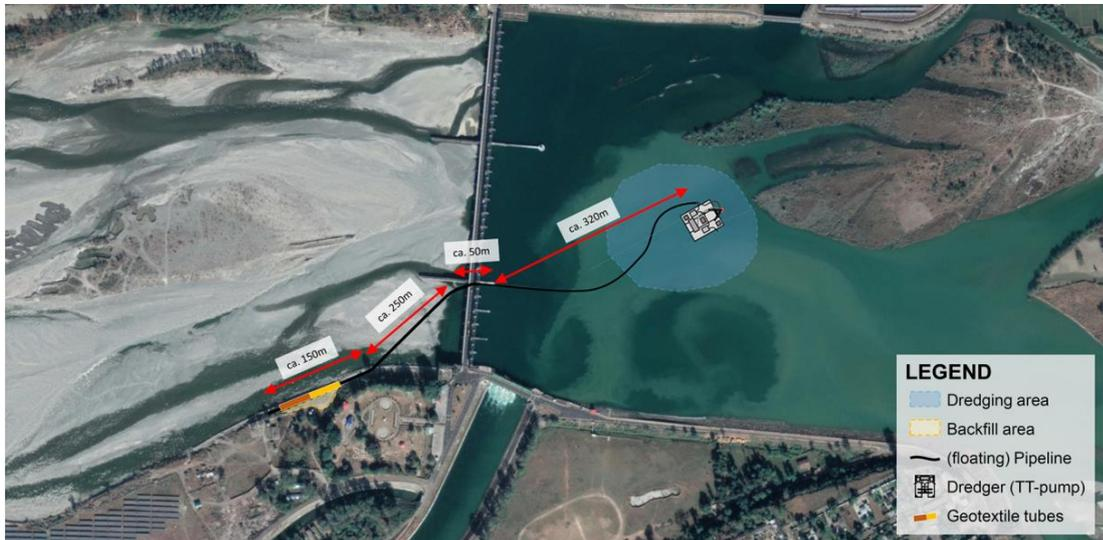
Figure 10 Dredging, transport and dumping arrangement.
