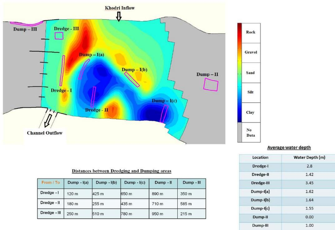
Figure 5 Dredging and dumping options in the Dakpathar Reservoir. The figure includes water depths at these locations and the distances from dredging to dumping locations.
