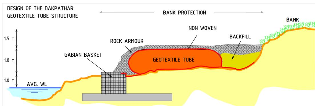
Figure 11 Design of bank protection structure using geotextile tube.
