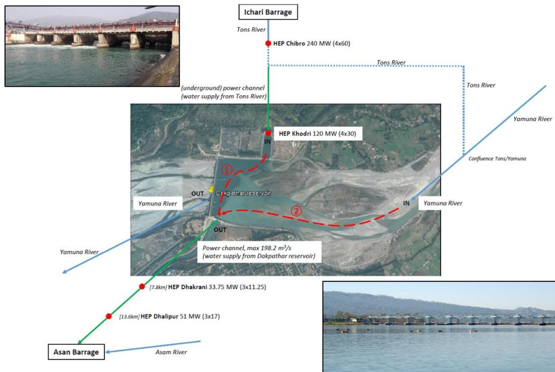
Figure 1 Overview of Dakpathar Dam. The figure includes two pictures. The upper one shows the downstream of the channel inlet while the lower picture shows Dakpathar Barrage and the upstream reservoir.
